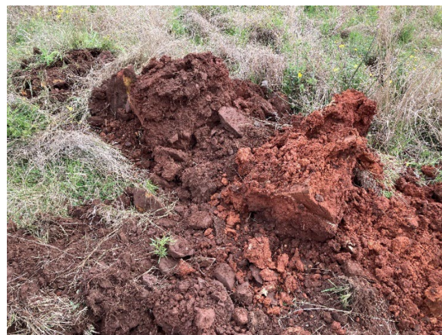
Photo 16 – Excavated soil showing high rock content
