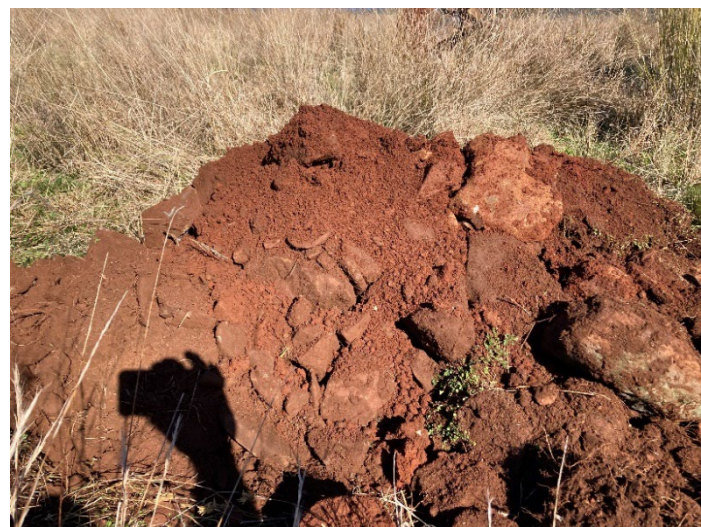
Photo 32 – Excavated Soil Material (Showing High Rock Content)
