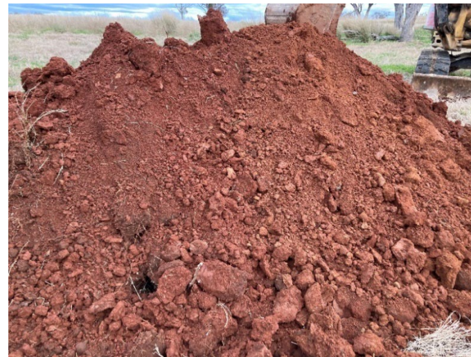
Photo 52 – Excavated Soil Profile showing Rock Throughout
