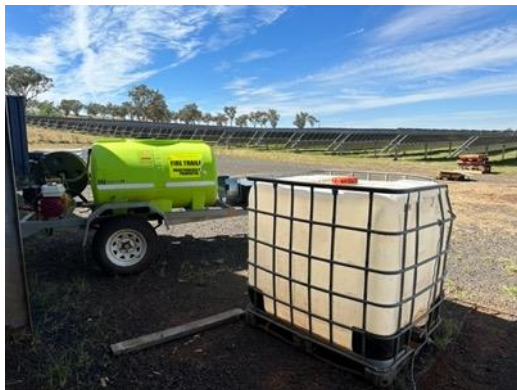
Photo 27: Portable firefighting trailer and water tank.
